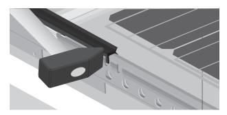
Both seal ends are fully pressed tightly against each other there and each fastened with a clamping lug.
