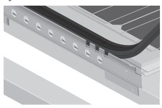
The transverse seal is to be measured in such a way that it extends over several modules. The transitions from module to module are each supported by using a transverse seal clip (see Figure 25 and Figure 26).
