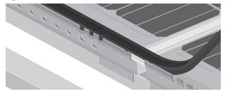
If a transverse seal (approx. 6.4 m) is not long enough within a module row, then it is to be shortened near its end so that the transition from one transverse seal to the next can be made in one of the two clamp areas per module each with two clamping lugs.
