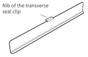
The remaining length of the transverse seal can be laid in the meantime on the last fitted module.
