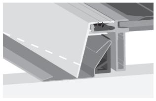
Cut for adaptation to roof-side gutters in lowest module row
