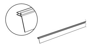
Module connection top long (Only for modules in right and left module field corner)
