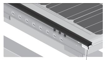
3 mm projection of the transverse seal over the transverse seal spacer
