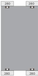
Max. permitted pressure load up to 1,067 Pa (test load 1,600 Pa)
