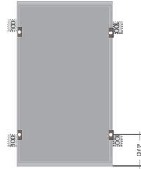
Max. permitted pressure load up to: 3,600 Pa (test load 5,400 Pa)
