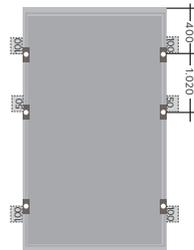
Max. permitted pressure load up to 3,600 Pa (test load 5,400 Pa)
