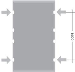
Max. permitted pressure load up to 2,400 Pa (test load 3,600 Pa)
