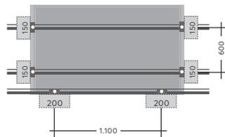
Max. recommended pressure load to the module: 5,400 N/m<sup>2</sup>
