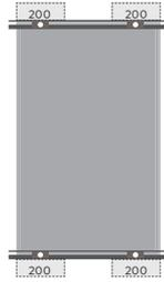
Max. recommended pressure load to the module: 2,400 N/m<sup>2</sup>
