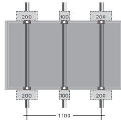
Max. recommended pressure load to the module: 5,400 N/m<sup>2</sup>
