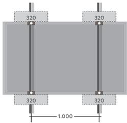
Max. recommended pressure load to the module: 2,800 N/m<sup>2</sup>
