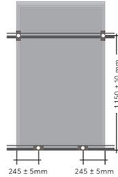
Max. recommended pressure load to the module: 3,600 N/m<sup>2</sup>
