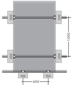
Max. recommended pressure load to the module: 5,400 N/m<sup>2</sup>
