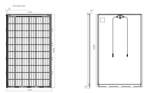
The roof construction must comply with the general requirements of the directives of the Central Association of the German Roofing Trade (ZVDH); the system is designed for **40 x 60 mm roof battens**.
