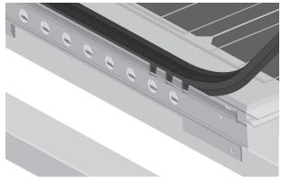
The transverse seal is to be measured in such a way that it extends over several modules. The transitions from module to module are each supported by using a transverse seal clip (see Figure 25 and Figure 26).
