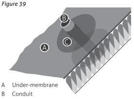
C Flexible system adhesive tape Connection of the steam brake/air-tight layer room side as shown.
