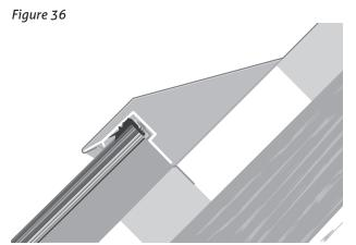
Now install the side roof enclosure frame.
