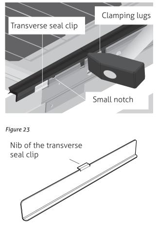
The remaining length of the transverse seal can be laid in the meantime on the last fitted module.
