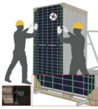
5. Fix the slipping-stop beam to the supporter base from the other side
