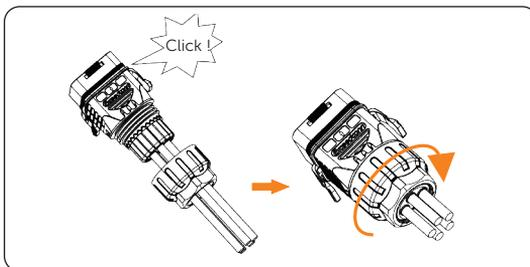
Figure 7-45 Assembly connector
