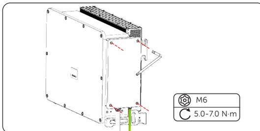
Figure 7-25 Closing the AC wiring box
