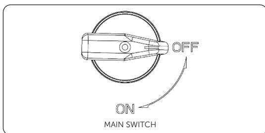
Figure 8-3 Turning off the main switch
