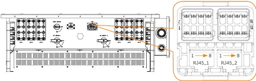
Figure 7-38 Communication port pin number
