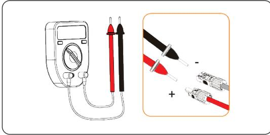
Figure 7-34 Measuring the voltage of PV connectors
