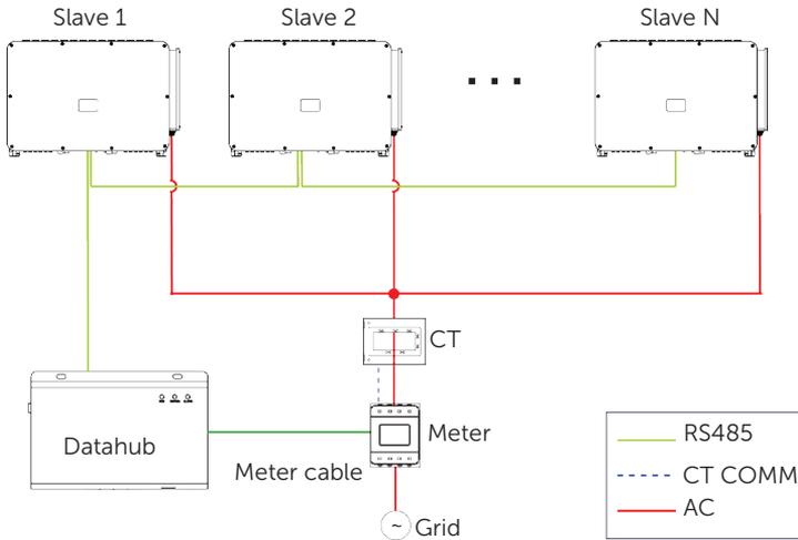
Figure 14-1 Parallel system diagram with Datahub
