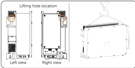
Figure 6-9 Crane handling
