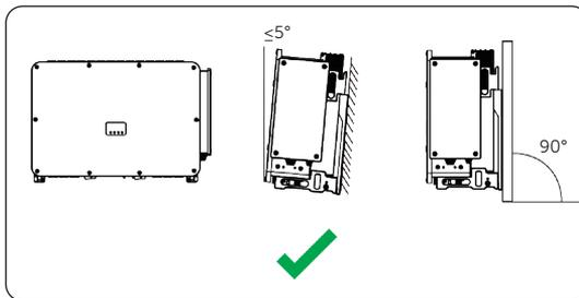
Figure 6-1 Correct installation
