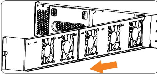
Figure 11-3 Pulling out the fan bracket completely
