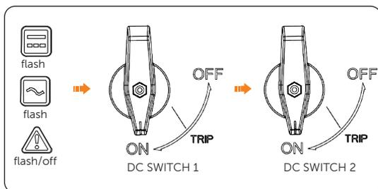
Figure 8-2 Turning on DC switches
