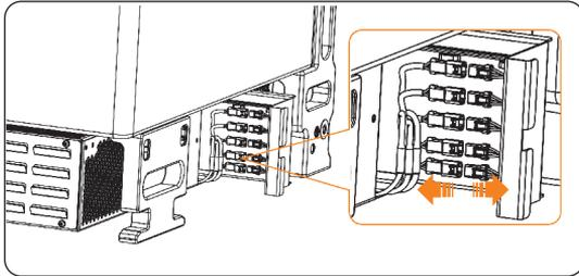
Figure 11-2 Disconnecting the cable
