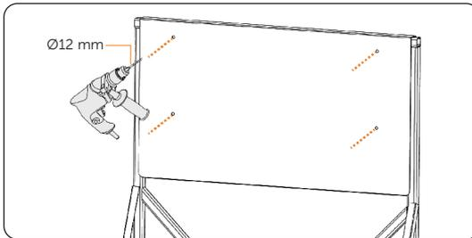
Figure 6-6 Drilling holes
