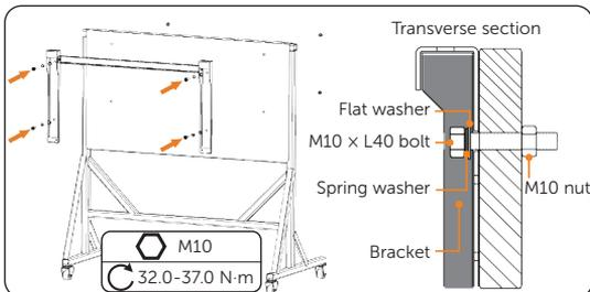
Figure 6-7 Securing the bracket
