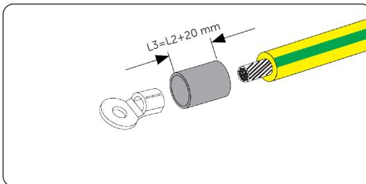
Figure 7-8 Installing the tubing and OT terminal
