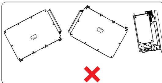
Figure 6-2 Incorrect installation
