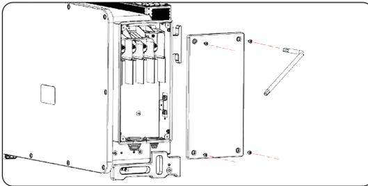
Figure 7-17 Opening the AC wiring box cover
