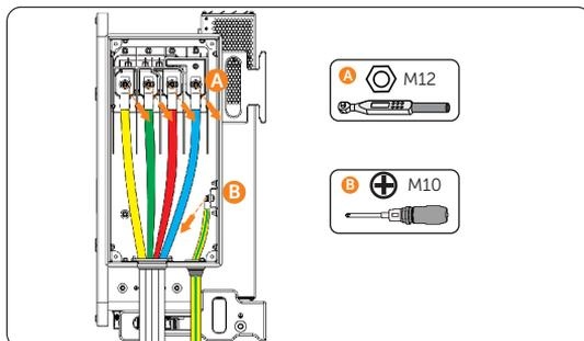
Figure 12-6 Disconnecting cables
