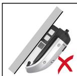
Do not install the inverter overhanging with the connections upwards.
