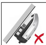
Do not install the inverter overhanging with the connections downwards.
