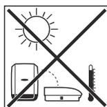
In order to keep inverter heating as low as possible, do not expose the inverter to direct sunlight. The inverter should be installed in a protected location, e.g., near the solar modules or under an overhanging roof.
