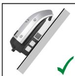
The inverter is suitable for installation on a sloping surface.
