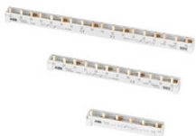
2CDL230002R1009 PS3/9-FI Phasenschiene 3Ph.,9Pins,10qmm,für FI
